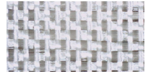
1080 Open-filament Glass Fiber
